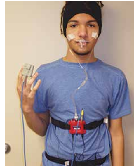
Figure 38: Level 3 HST setup
