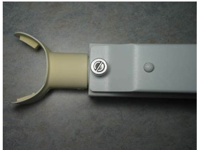
Fig. 3 Using a scalpel, the lingual tab was removed from the mouthpiece, which was then used for acoustic pharyngometry
